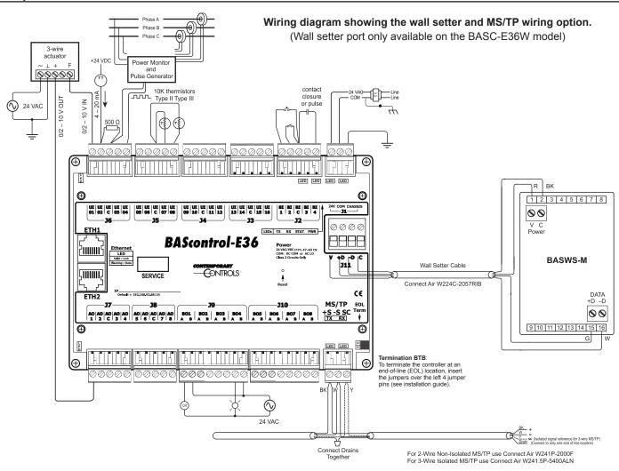
To enable or disable bias/termination, install jumpers as shown.
